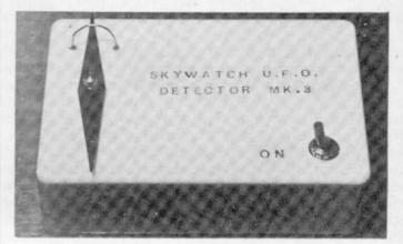
A magnetic needle type detector incorporating a solid state latching circuit for the audio alarm. Battery operated.
